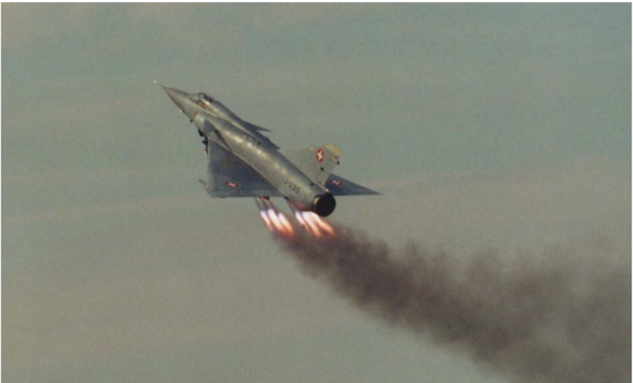
A Swiss Air Force Mirage IIIS during a JATO takeoff! (photo via wikipedia)
