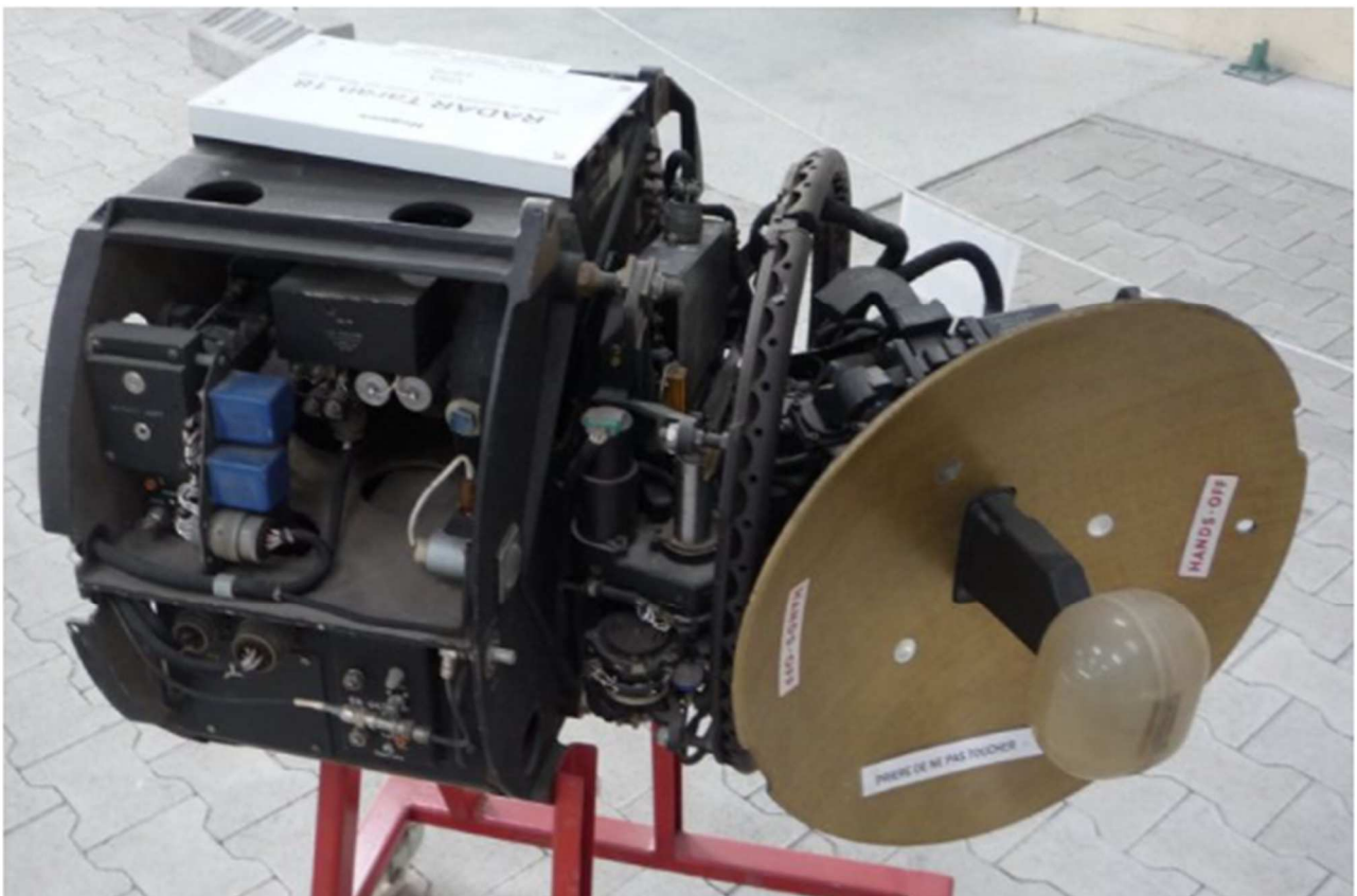
A Hughes TARAN 18 radar from a Swiss Mirage IIIS. (image via Wikipedia)
